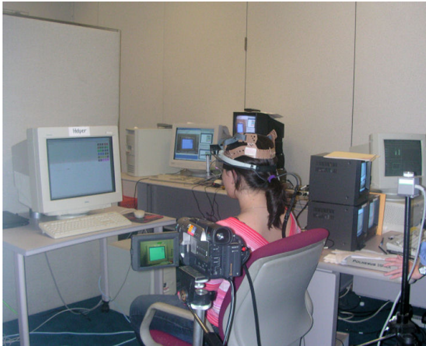
Figure 2.13: Setup for gaze based action prediction and camera control. Image taken from [OOF + 05].
